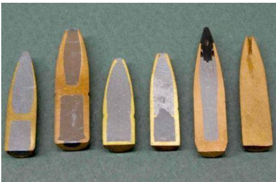
Figure 7: Cross sections of some bullets used for hunting purposes depicting the different designs regarding material, shape and jacketing (Source: Wikimedia Commons).
