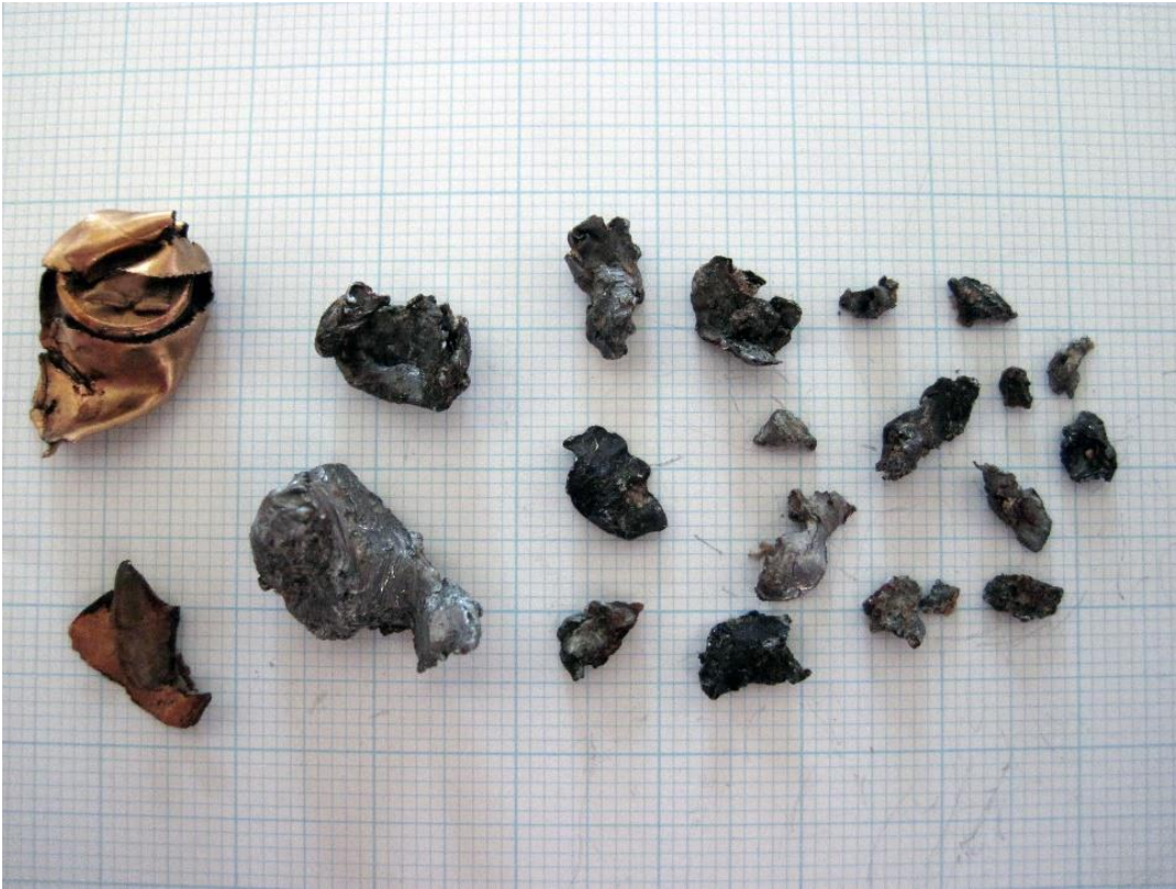
Figure 22: Fragments from a deforming bullet retrieved from a carcass. Note the main fragment (bottom of the projectile) on the upper left (Source and © FIWI).
