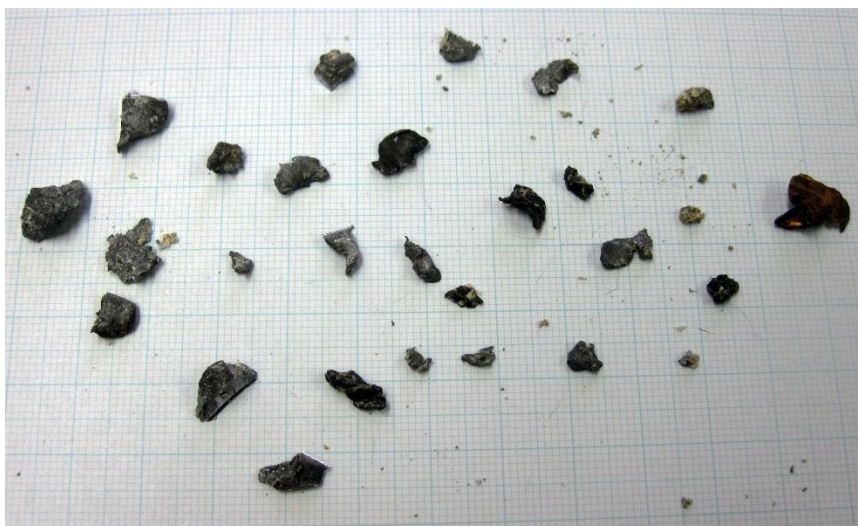
Figure 9: Fragments of a disintegrated frangible bullet that is found along the wound path in the carcass (Source and © FIWI)
