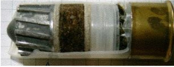
Figure 11: Cross section of a shotgun shell containing a slug (at left) (Source: Wikimedia Commons).
