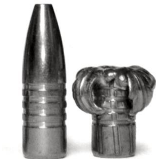
Figure 8: The shape of a deforming bullet before (left) and after hitting a body (right). Note the typical “mushroom shape” that ensures high energy-transfer in the body (Source: Internet).
