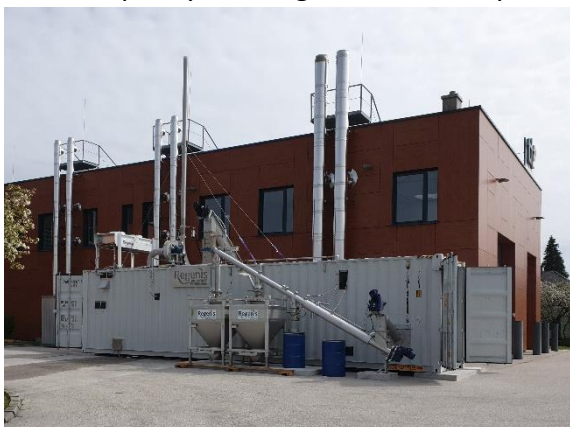
Figure 3: left: Pilot Scale pyrolysis plant from outside; right: pyrolysis plant inside container, pyrolysis reactor on left and gas burner on right side
