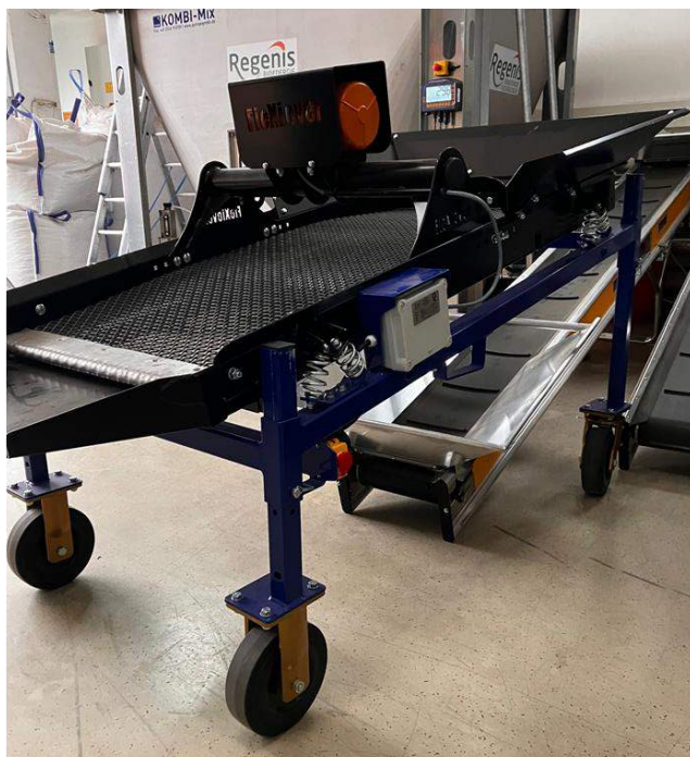
Figure 2: The 16x16 mm sieve apparatus made by FleXiever located at BEST, used to sieve sample 10
