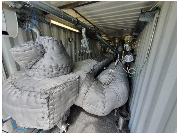
Figure 3: left: Pilot Scale pyrolysis plant from outside; right: pyrolysis plant inside container, pyrolysis reactor on left and gas burner on right side
