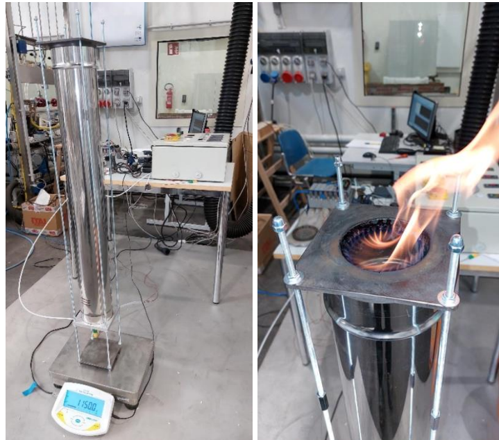
Figure 2: Lab-scale gasifier – mounted on weighing scale (L), during operation (R)
