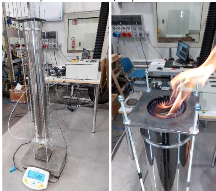
Figure 2: Lab-scale gasifier – mounted on weighing scale (L), during operation (R)
