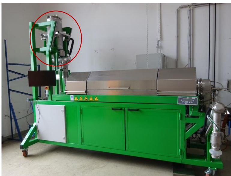
Figure 2: The used rotary kiln system, with the feedstock storage marked in red.
