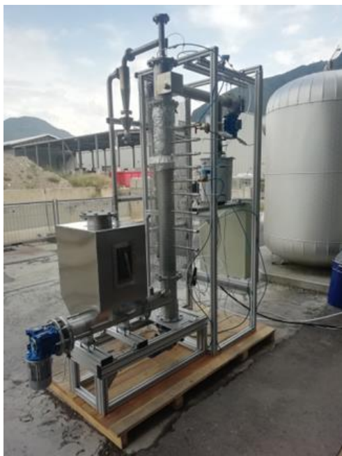
Figure 3: Pilot scale gasification setup
