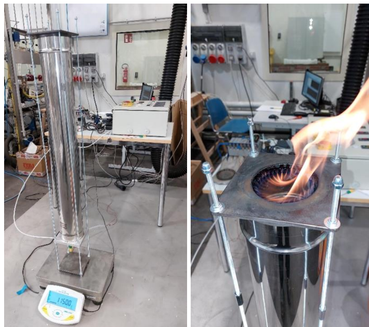
Figure 13: Lab-scale gasifier – mounted on weighing scale (L), during operation (R)
