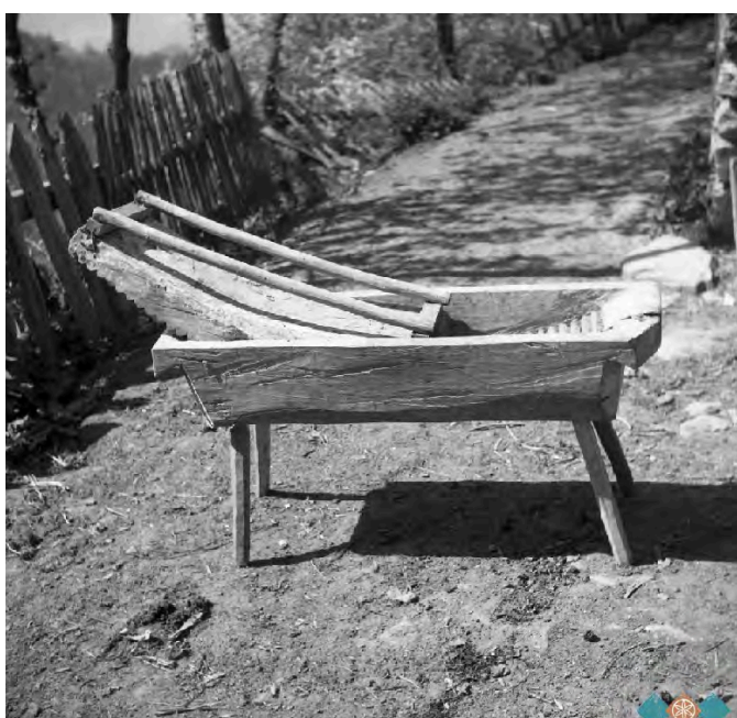
Simple device for fulling or walking from Slovenia. Source: Slovenski etnografski muzej
