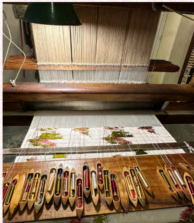
Shuttles of silk threads in colors allow to create a complex pattern. Foto: Verena Gruber.
