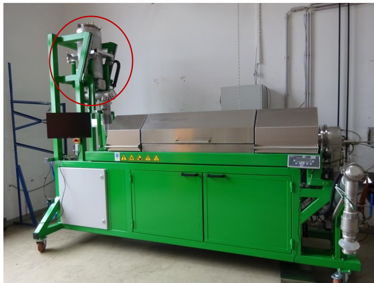
Figure 2: The used rotary kiln system, with the feedstock storage marked in red.
