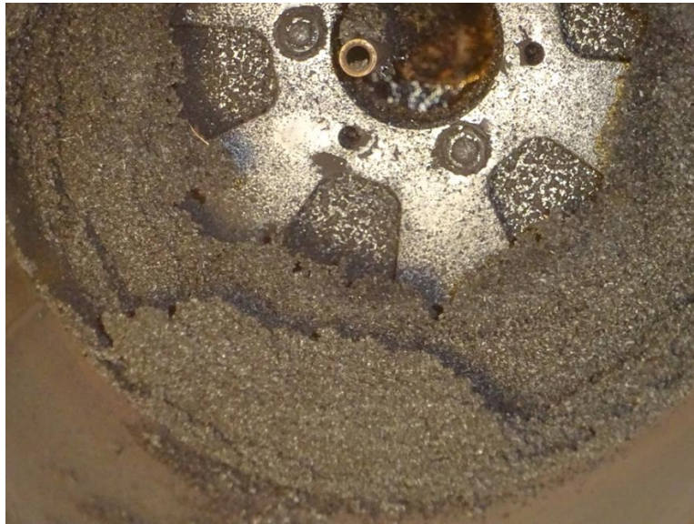
Figure 5: A picture of the reactor inside, taken from the exit of the drum. It represents the beginning of the heated reactor zone, where clearly visible the bran biochar accumulated
