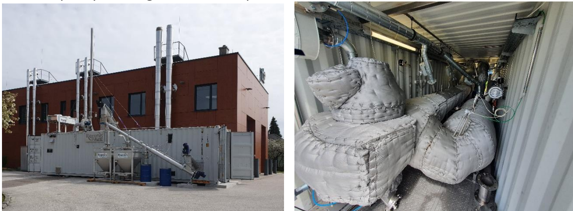
Figure 3: left: Pilot Scale pyrolysis plant from outside; right: pyrolysis plant inside container, pyrolysis reactor on left and gas burner on right side
