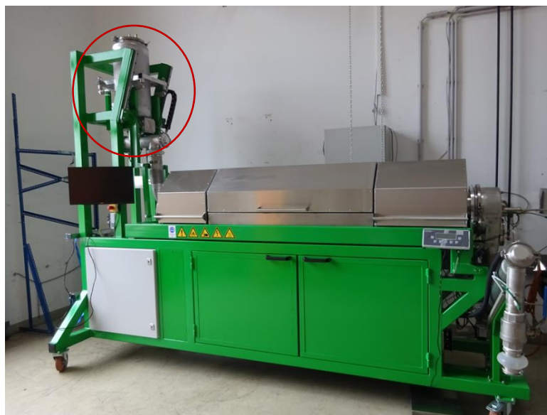
Figure 4: The used rotary kiln system, with the residue storage marked in red.
