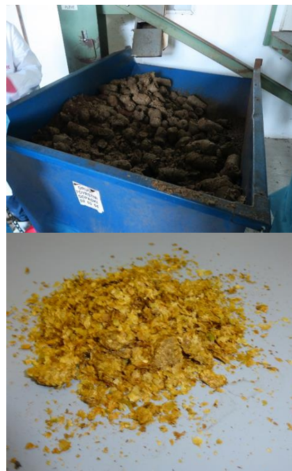
Figure 3: Top: The coffee husks in their final form after processing; Bottom: The second batch of coffee husks at BEST, set for pyrolysis
